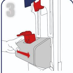
Slide the housing to the side to remove it. Slide the new housing into the slides, attach the belt buckle, and close the rear cover.
