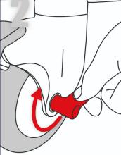
**Speed control** Turn the handle clockwise to limit the speed of movement.
