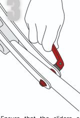
Ensure that the sliders are securely engaged in the safety grooves and tighten the levers on the sides.
