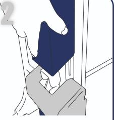
Lift the rear cover and detach the buckle between the housing and the belt.
