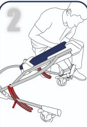
Loosen the levers on the sides and unfold the upper frame.
