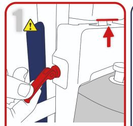
Lift the harness completely and firmly lock the brakes.
