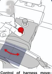
Control of harness movements on the transverse plane
